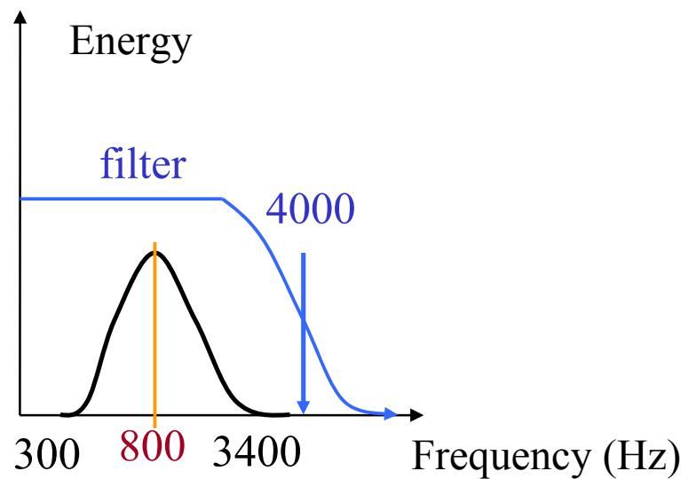
Cut off frequency of filter is at 4000 Hz
