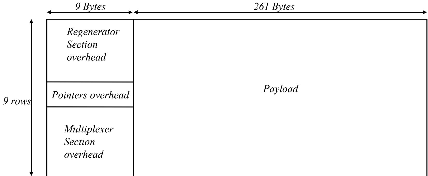
STM-1 : Synchronous transfer module
