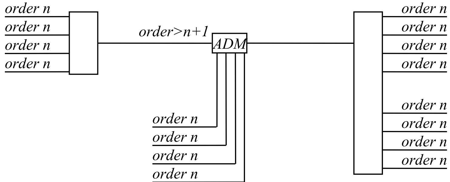
The condition : synchronous multiplexing
